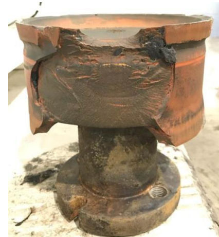
Damage Piston Pump Ram
