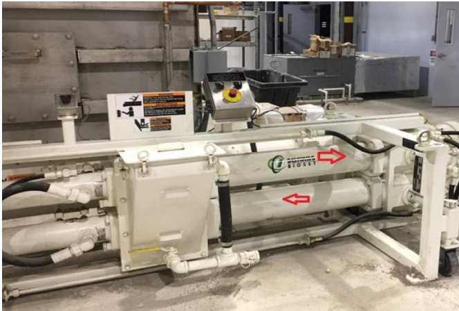
Location of Damaged Piston Pump Rams (Red Arrows)
